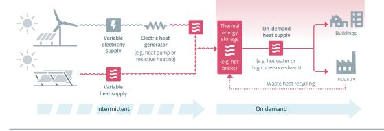
Thermal energy storage (TES) captures different intermittent energy sources as heat up to 1500°C. The stored heat is then available on demand for various applications.
