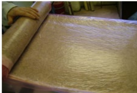
Figuur 14: hennep sheet moulding compound 16
