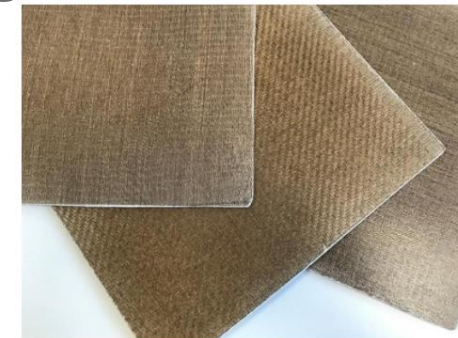
Natural fiber organic sheets made of flax fiber and Polyvertec 3830 (Source: Schill + Seilacher)
