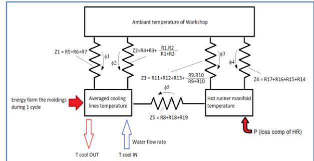
Fig. 05 : Thermal resistance network model.
