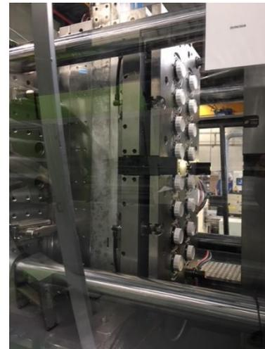
Fig. 06 : 16 cavities cap mold (courtesy of United Caps).
