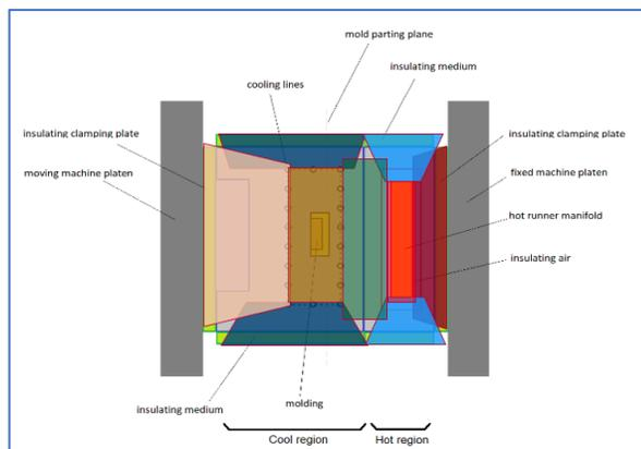
Fig. 02 : Divisions of an injection molding tool in several subregions.
