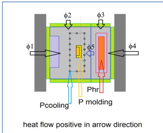
Fig.04 : Heat flows in the mold and positive orientations.
