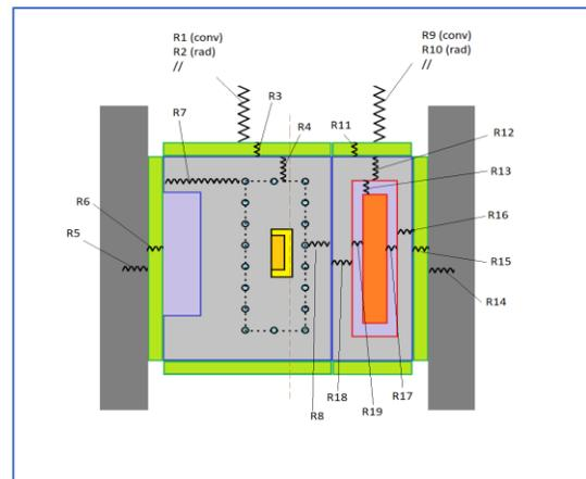
Fig. 03 : Model of thermal resistances.
