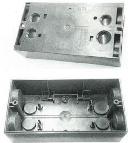
Fig. 08: PC housing base (ex. from “Gastrow – Injection Molds – 2<sup>nd</sup> ed. – 108 proven design – p.164)
