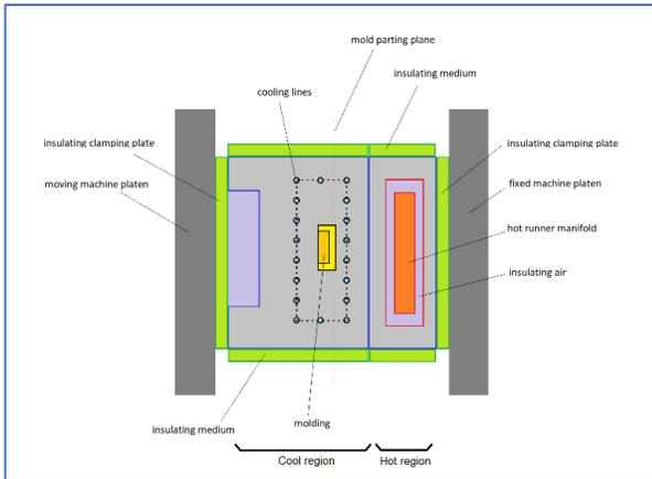
Fig.01 : Main parts of an injection molding tool.
