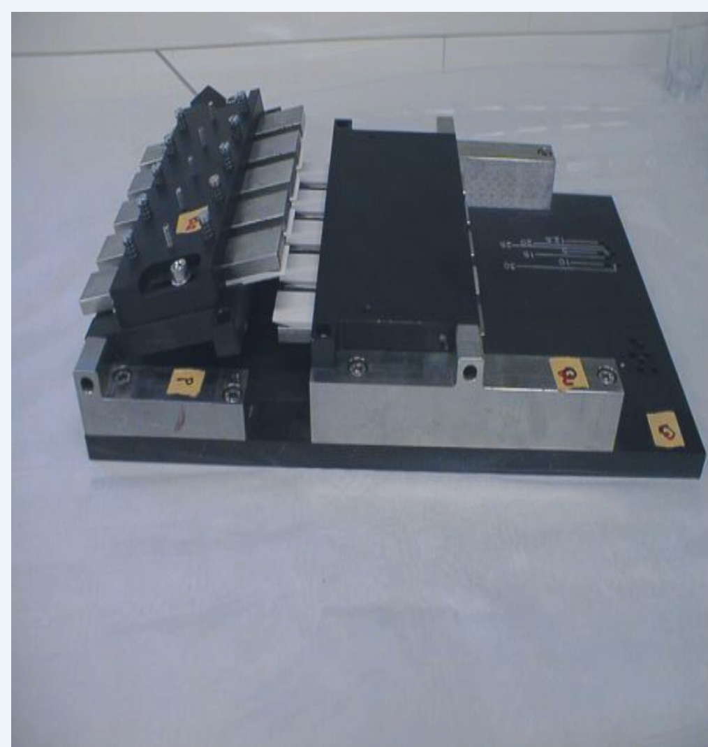
Device allowing joint thickness and overlap length control
