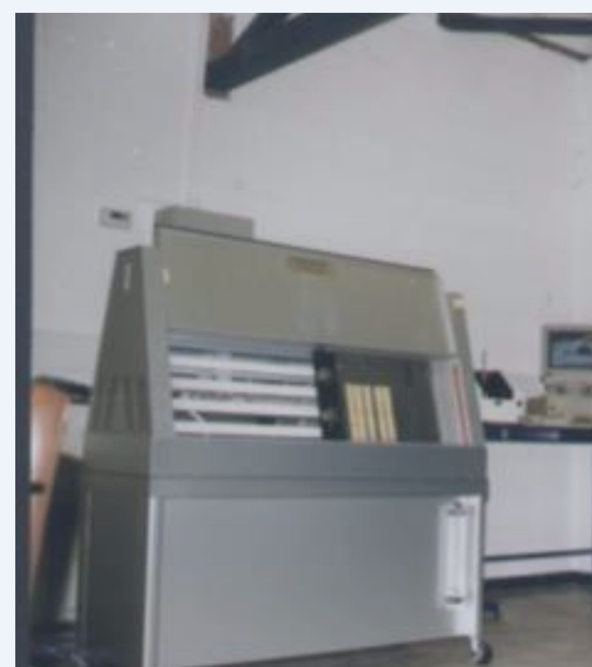
UVA 340 and UVB 313 ASTM D4329 – ISO 4892 ASTM G154
