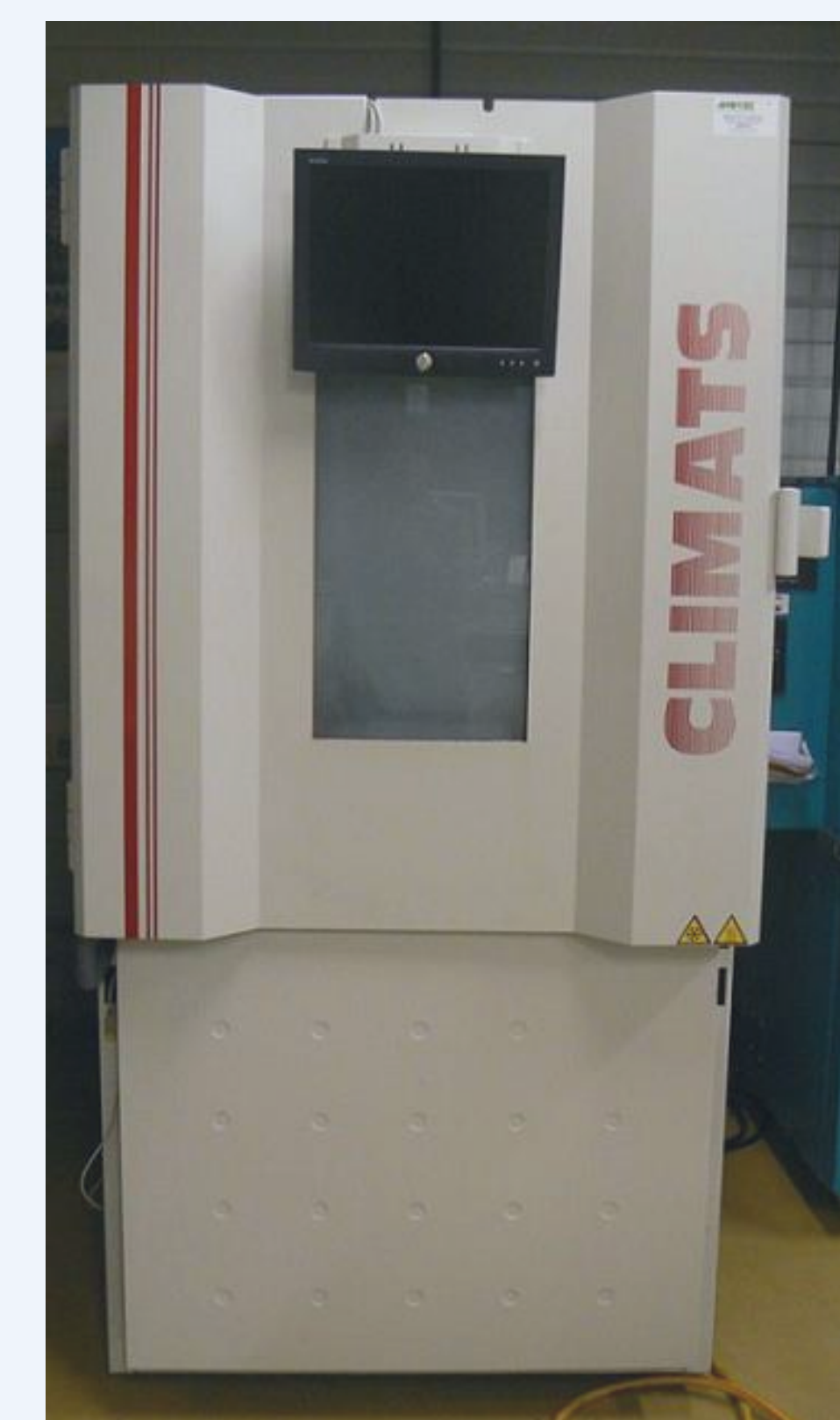
Climatic chamber -40°C to 150°C ISO 9142
