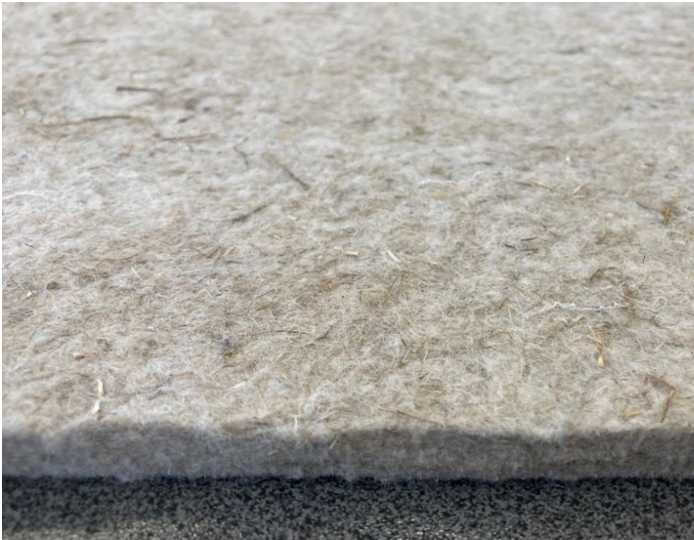
Figure 6: example of a non-woven mat in which the natural fibre and polymer fibre have already been pre-mixed
