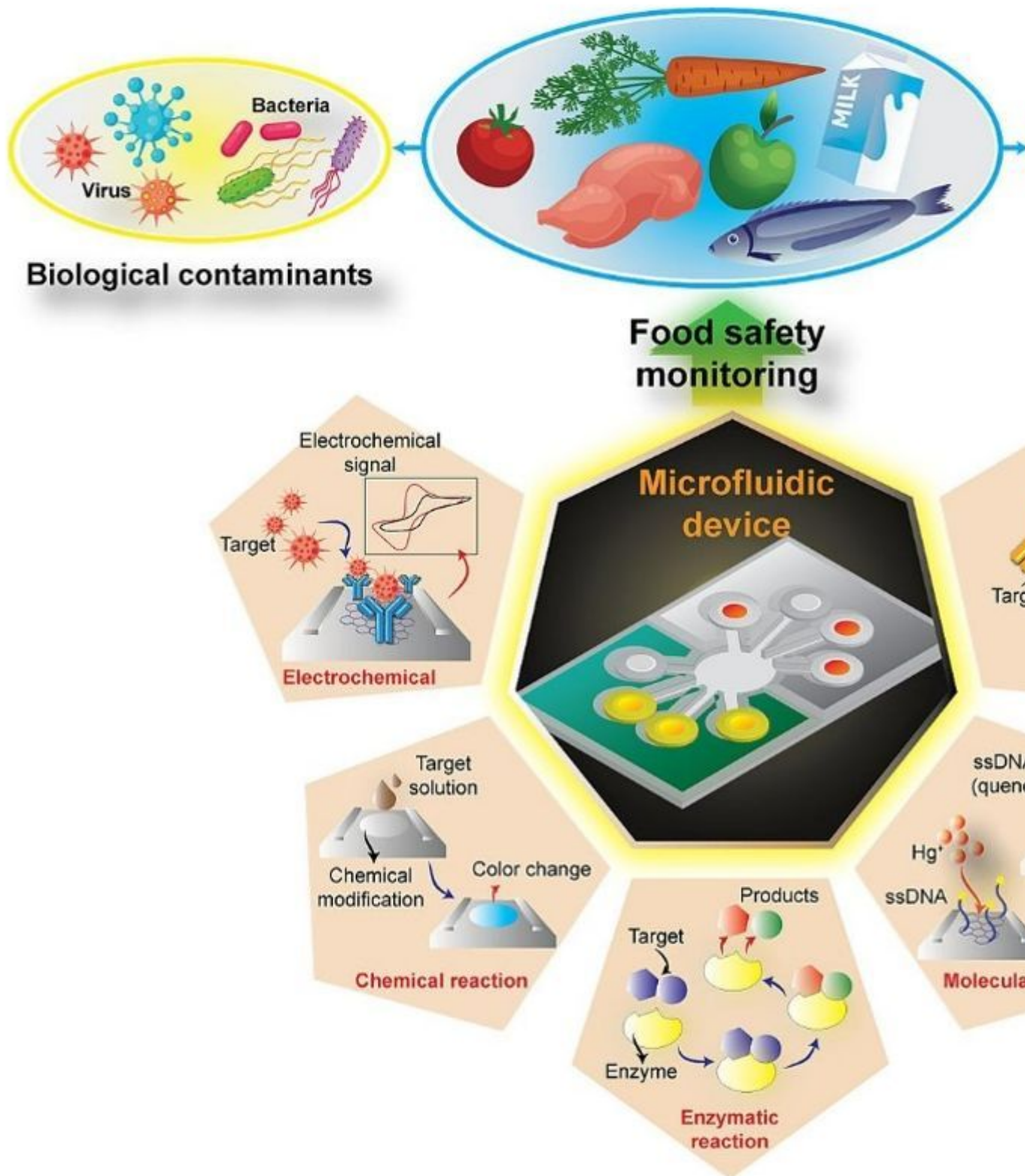
Figure 2 Microfluidic advances in food safety control (Source: Thi Ngoc Diep Trinh, Kieu The Loan Trinh, Nae Yoon Lee, Microfluidic advances in food safety control, Food Research International, Volume 176, 2024, 113799, ISSN 0963-9969, https://doi.org/10.1016/j.foodres.2023.113799 )
