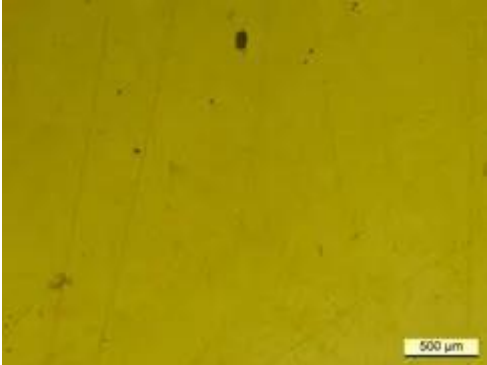
Figure 1: High density of the as-built state
