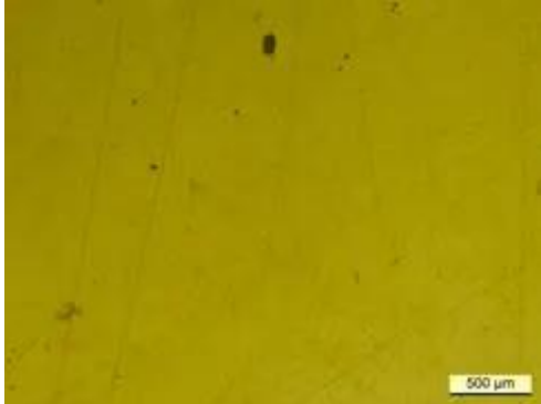
Figure 1: High density of the as-built state
