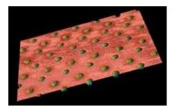
By means of a matrix of microscopic lenses, the light can be distributed according to need. This lens structure can be made by injecting the lens material into a mould with the right microstructures. In order to achieve this, a mould is processed with a femtosecond laser.
