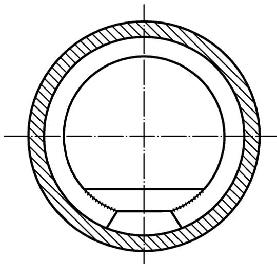
Figure 9.1-1 — Internal stiffening rings with a reinforced cut-out
