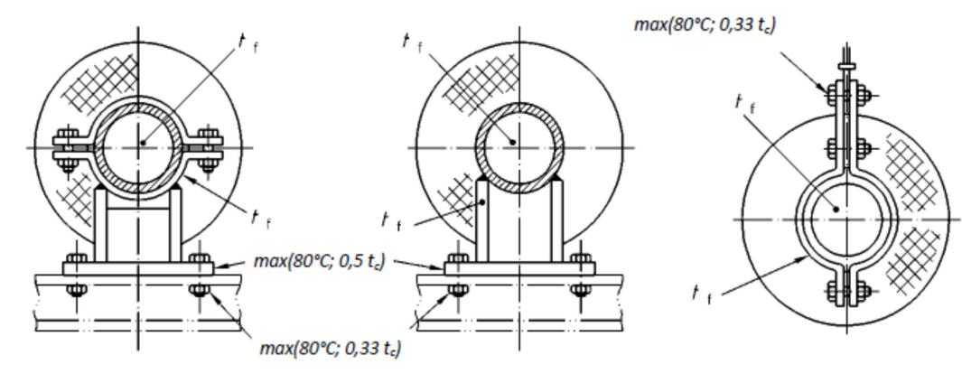
**Figure 13.11.2-1 — Support design temperatures inside and outside insulation**
