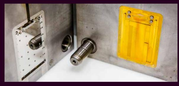
Prototype mould with exchangeable inserts
