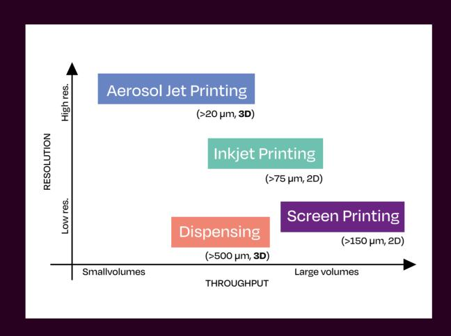
Selective material deposition at micro-scale on 2D and 3D substrates
